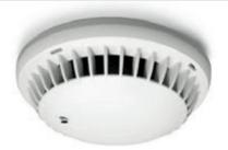
Optical smoke detector for loop3000 with 2 optical and 1 thermal sensor for earliest fire detection and indication and with bidirectional isolator according to EN 54-7 and EN 54-17.
