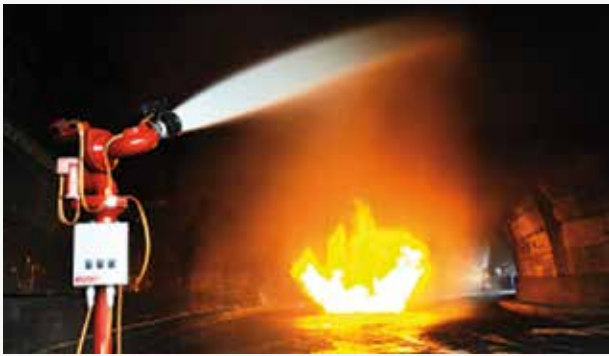
Motorway Tunnel in Montelibretti (pool fire)
