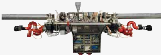
Picture of the mobile unit (monitors on trailer) with the demounted external covering.
